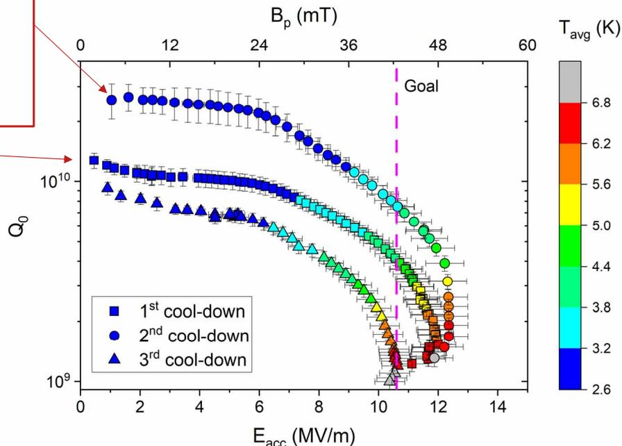
$T_{\text{avg}}$  is the average cavity temperature, cooled by cryocoolers
