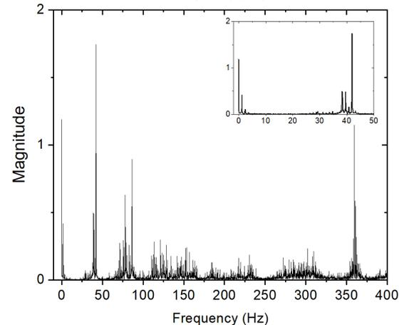
*FFT of cavity frequency shift*
