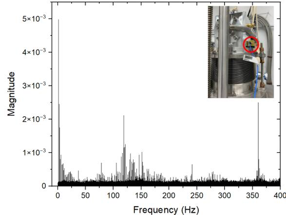
*FFT of vertical component of acceleration*
