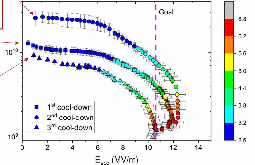
$T_{avg}$  is the average cavity temperature, cooled by cryocoolers
