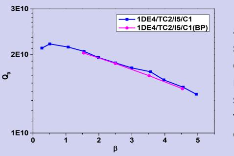
All inserts at AMTF have an additional relay box, which is used to select the RF loops during cable calibration. Both of the curves with normal (blue) and bypass (pink) setting act in the same way, hence the relay box can be excluded as error source.
