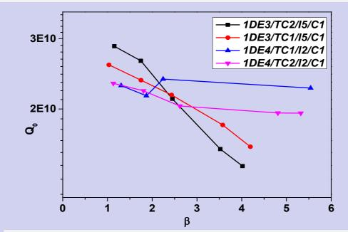
For both cryostat, the results were that 1DE3 with Insert 5 shows a dependency of  $\beta$  (black and red) while 1DE4 in Insert 2 (blue and pink) shows an independency, which means both RF and cryostat systems are working well.
