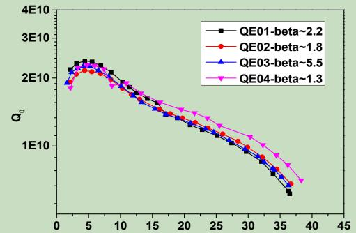
In principle, the curves from the same vertical test should the be same. According to earlier research of cavity performance at **DESY**, the measurement error Q is around 10% (maximum less than 20%).
