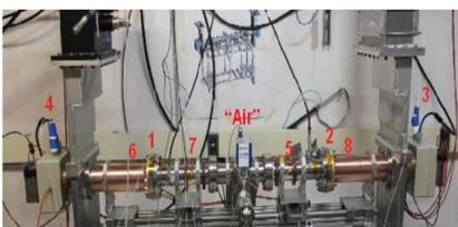
Full assembly on test stand support. Pumping, diagnostics, air cooling system. 8 T-sensors to control temperature of coupler and cooling air
