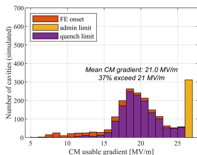
*Simulation of LCLS-II-HE cryomodule gradients with improved vertical test gradients but the same multipacting and field emission rates as in LCLS-II*
