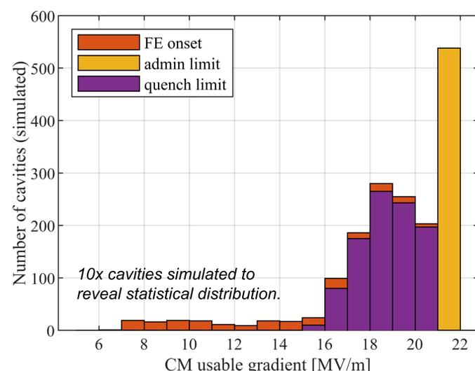
Peak vertical test accelerating gradients of LCLS-II cavities are well fitted by a two-parameter **thermal defect model**.
