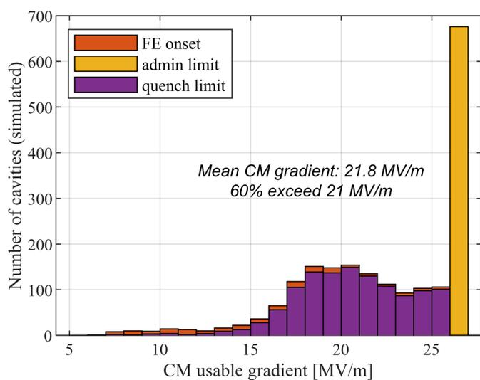
*Simulation of LCLS-II-HE cryomodule gradients with improved vertical test gradients and rates of multipacting and field emission decreased by 50%*
