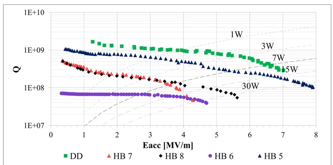
Fig 4: Q-slope of the ALPI QWRs.
