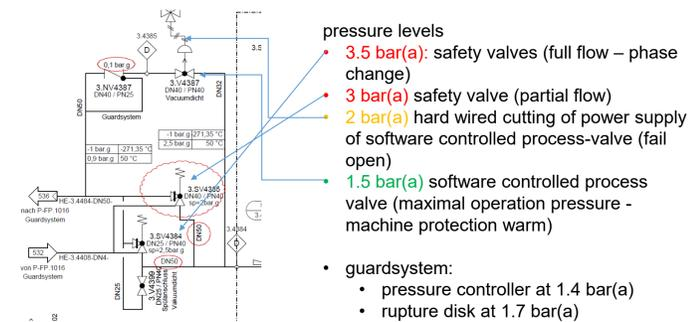
Due to space restrains on the possible sites it was not possible to integrate safety valves inside the module. Therefore, they had to be integrated in the feedbox.
