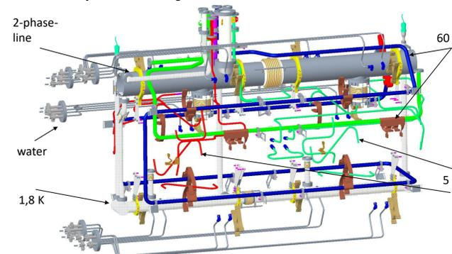
The 5 K and 60 K circuits are operated supercritical at 3 bara and 12 bara. The components are all supplied with serial piping.
