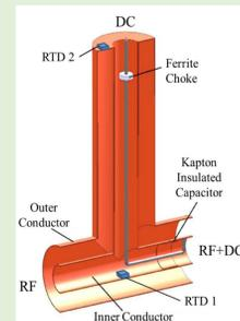
The design was iterated several times to reduce the heating on the inner conductor when operating at high power (5 kW).
