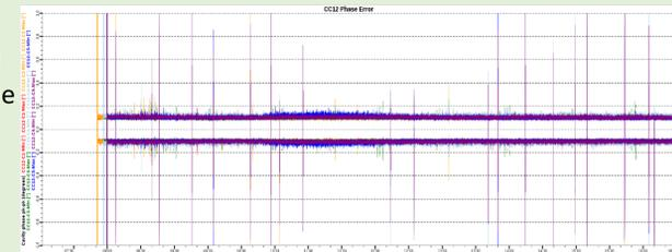
Correlated phase jumps in the last  $\beta=0.29$  cryomodule.
