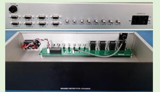
Spark detector chassis in the rack room.
