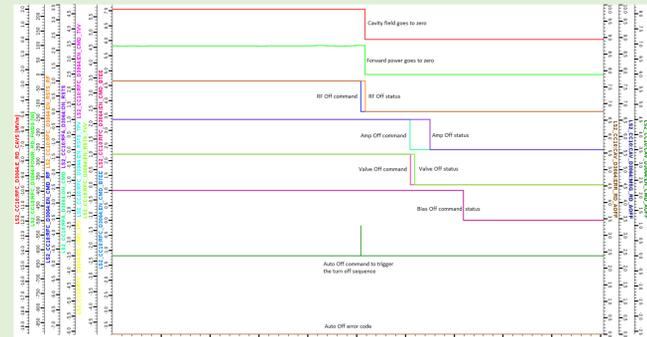
An HWR cavity auto off sequence.
