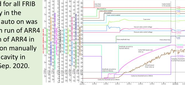
An HWR cavity turned on automatically and locked in 35 seconds.
