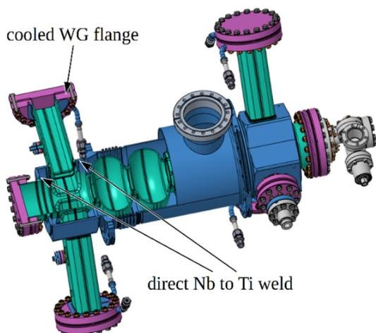
Figure 5: Cavity with ancillaries for cold test (Nb structure in green, NbTi flanges in pink and Ti parts in blue).
