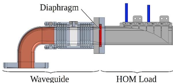
Figure 8: Waveguide with HOM load and diaphragm.
