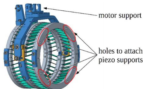
Figure 6: Blade tuner model with leverage.
