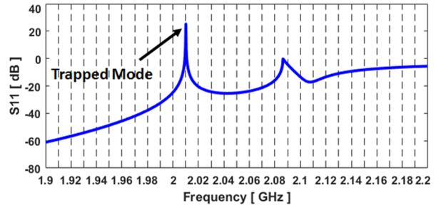
Figure 4: Reflection coefficient of the bellow for the TM mode excitation at the beampipe port.
