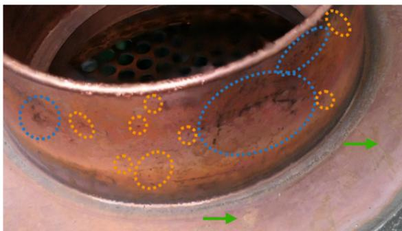
Figure 11: CsB inner labyrinth after cutting the bellow.
