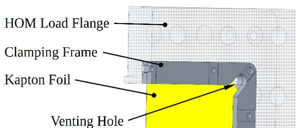
Figure 9: Detail of the diaphragm and its support frame. Venting holes in each corner also avoid creases in the foil.
