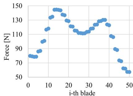
Figure 7: Force distribution on the 50 blades displayed for one tuner ring with 5 kN applied.
