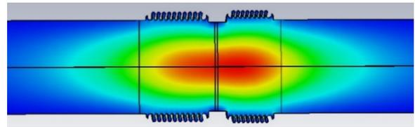
Figure 3: Electric field of the bellow's trapped resonant mode ( $f = 2010$  MHz,  $R/Q = 0.74 \Omega$ ,  $Q = 1960$ ).
