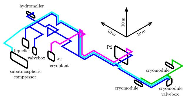
Figure 3: Piping path for connecting the cryoplant hall above ground with the accelerator hall below ground. The old building structure is limiting the possible paths [9]. Dark blue represents the liquefier connection to the cryomodules valve box and P2 solenoid, green the distribution from the cryomodule valve box to the modules, light blue the 16 mbar string and magenta the P2 target cooling circuit.
