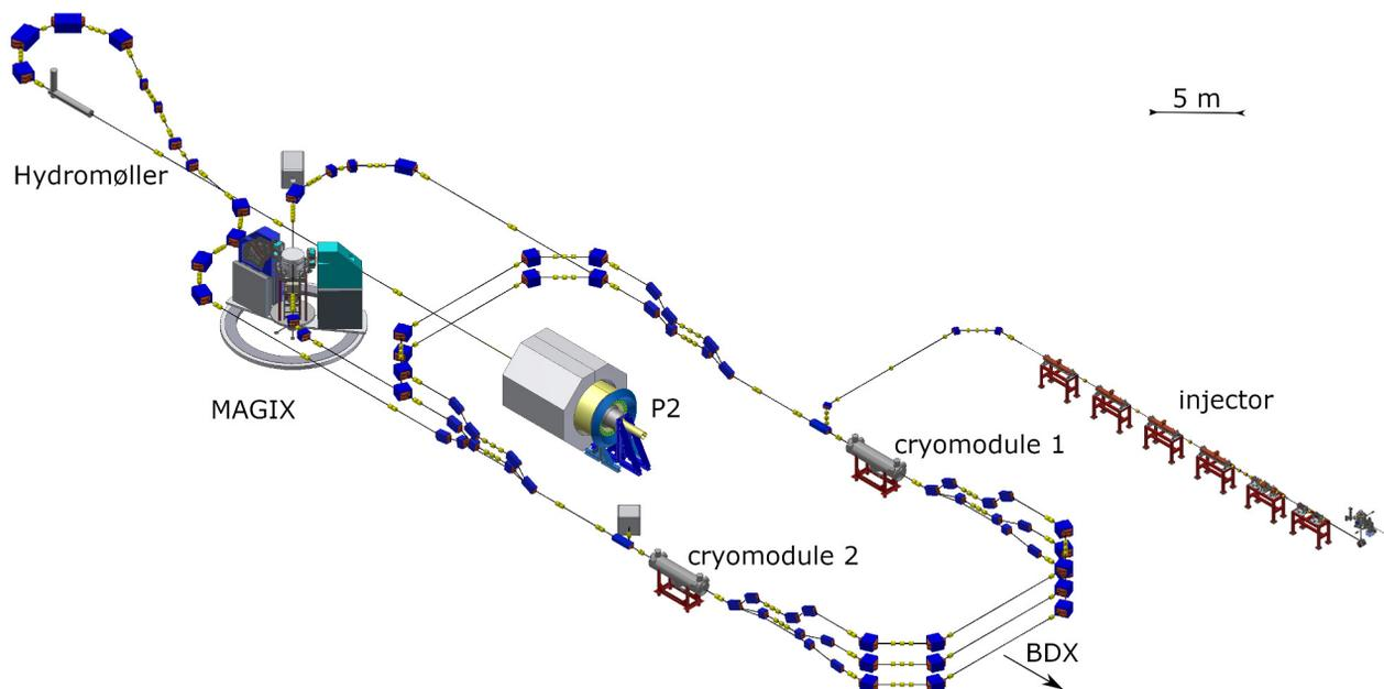
Figure 1: MESA lattice. Electrons are produced and pre-accelerated to 5 MeV in the injector before they are injected into the recirculating main-accelerator. The cryogenic components are the P2 experiment (solenoid and target), the hydromøller for polarization measurements, as well as the cryomodules. The BDX experiment is positioned outside of the accelerator hall, but in line with the P2 beam dump and not shown in this picture.
