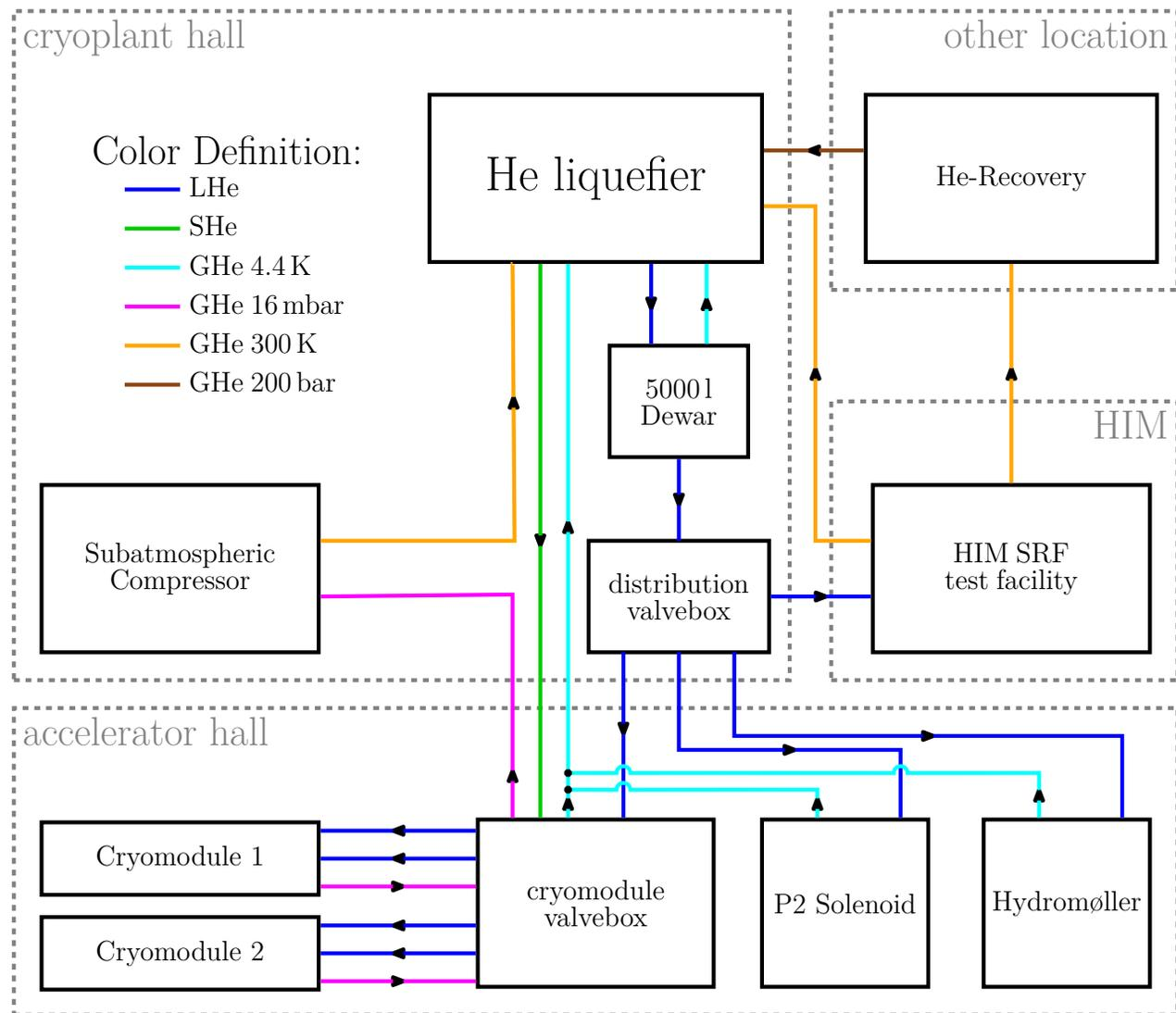
Figure 2: Process Flow Diagram (PFD) of the cryogenic distribution layout for MESA. The accelerator components to be supplied with liquid helium (LHe) are located in the accelerator hall. In addition, the SRF test area of the Helmholtz Institute Mainz must be supplied. A supercritical line (SHe) is foreseen, which also serves for a controlled cooldown. The gaseous phases (GHe) are color-coded according to their temperatures (light blue and orange) and pressures (magenta and brown).
