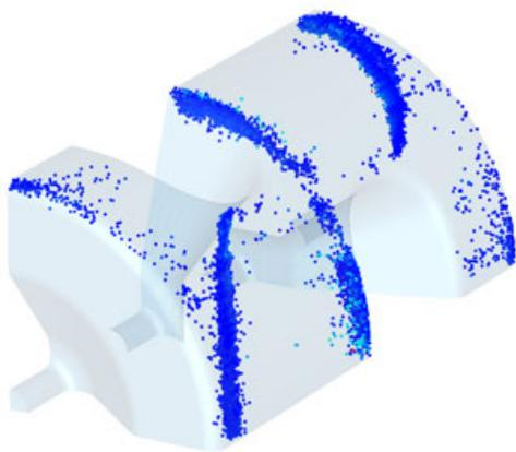
Figure 3: The secondary electron trajectories of the 2<sup>nd</sup> and higher order MP barriers. The displayed results are combined data from 0.5 MV/m to 2.8 MV/m.
