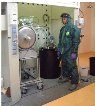
Figure 1: Chemical treatment system equipped with a single Spoke resonator currently used at IJCLab.
