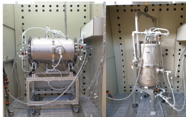
Figure 2: ESS cavity in horizontal and vertical position.
