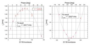
Figure 3: Example of measured  $f_s$  as a function of scale of trombone-type phase shifter of the target cavity.  $f_{s.max}$  and  $f_{s.min}$  from the fit results are also shown.
