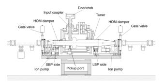
Figure 1: Cross-sectional view of the SCC module of SuperKEKB.
