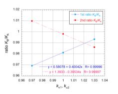
Figure 4: Ratio of the calibration factors of Group B ( $K_B$ ) to Group A ( $K_A$ ) as a function of  $k_{\alpha 1}$  or  $k_{\alpha 2}$ . Linear fit results as a function of  $k_{\alpha 1}$  or  $k_{\alpha 2}$  are also shown.
