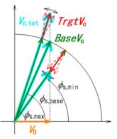
Figure 2: Schematic view of  $V_c$  calibration method by measurement of  $f_s$ . *BaseV*<sub>c</sub> is vector sum of four base cavities. The *TrgtV*<sub>c</sub> is the cavity voltage of a target cavity of the calibration.  $V_{c.tot}$  is vector sum of *BaseV*<sub>c</sub> and *TrgtV*<sub>c</sub>.
