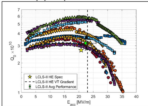
Figure 3: Cavity test results from proposed JLab recipe.
