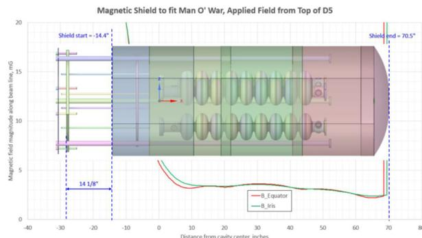
Figure 5: Dewar magnetic field simulation (G. Cheng).
