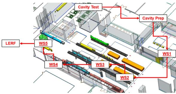
Figure 7: Layout of the Test Lab.
