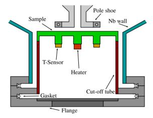
Figure 2: Cross-sectional view of the calorimetry chamber [15].
