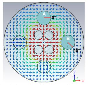
Figure 9: Cutting plane of the QPR normal to the z-axis. The input antenna loop area was fixed at 0° in port position A and the probe oriented at 45° in B. The magnetic field distribution corresponds to a quadrupole mode.
