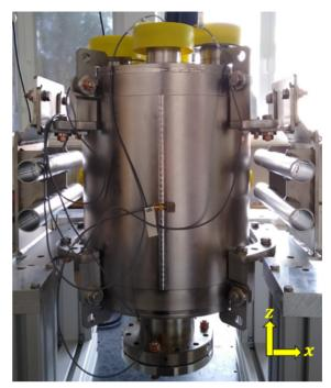
Figure 6: Mechanical resonances setup: four piezoelectric accelerometers mounted on the QPR's surface to measure vibrations in the x, y, and z axes.
