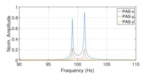
Figure 7: Normalized fast Fourier transform vs. Frequency. Three piezoelectric accelerometers (PAS) mounted on the top part of the QPR measured vibrations in the three dimensions when hitting it in the vicinity of the sensors.
