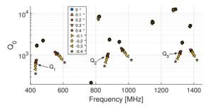
Figure 4: Quality factor vs. Frequency of the QPR at room temperature with a rotation of the rods around the *y*-axis at an angle  $\theta$  between -0.4° and 0.4°.
