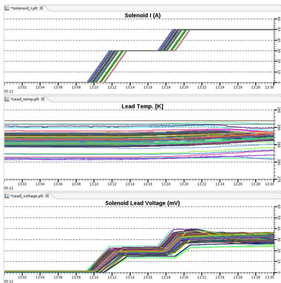
Figure 6: All 69 solenoid packages auto turn-on details in FRIB tunnel.
