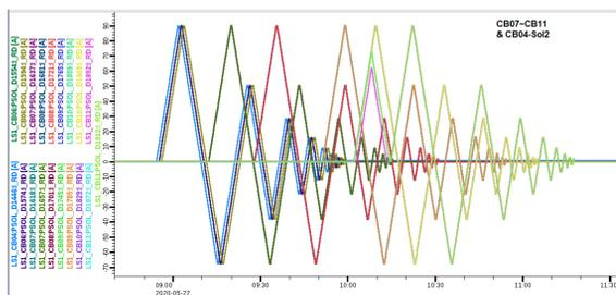
Figure 7: Solenoids automatic degaussing.
