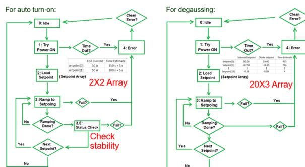
Figure 1: Solenoid auto turn-on and degaussing state-chart.
