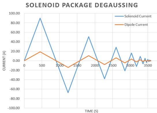
Figure 2: The simulated plot for the solenoid package degaussing procedure with 20 set-point current setting.
