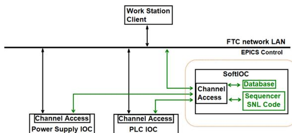
Figure 8: The IOC level program implement schematic.
