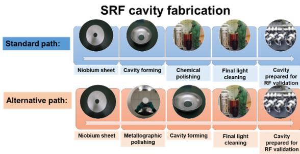
Figure 3: Sketch of the cavity fabrication.
