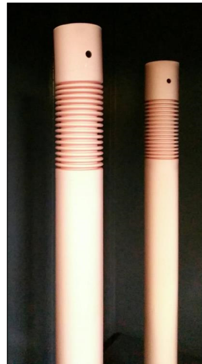
Warm IC: 150um copper plating Very difficult!
