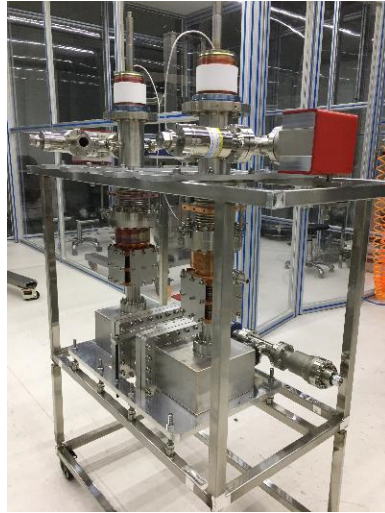
Clean assembly and vacuum leak check
