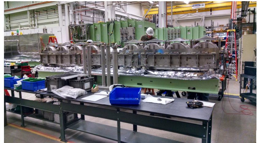
Coldmass Assembly Installed to Baseplate
