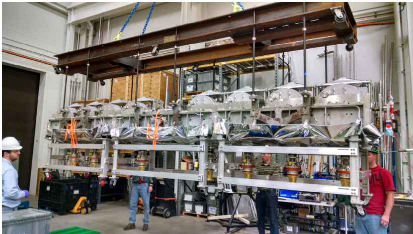
Coldmass Assembly Lifted to Baseplate
