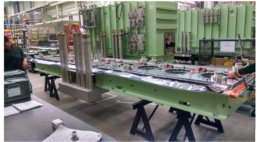
Cryomodule Baseplate Prepared
