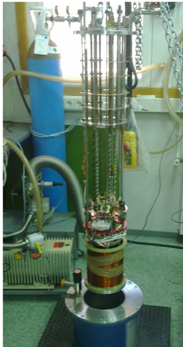
Qualification of the coils and integration in the helium vessel.
