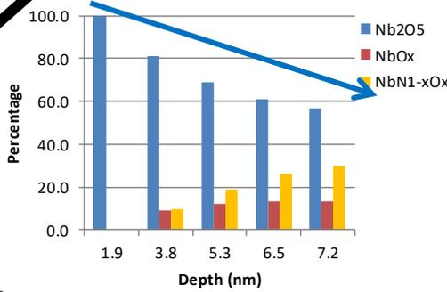
**NbN<sub>1-x</sub>O<sub>x</sub> is found on Nb baked at 140-160°C in N atmosphere**
