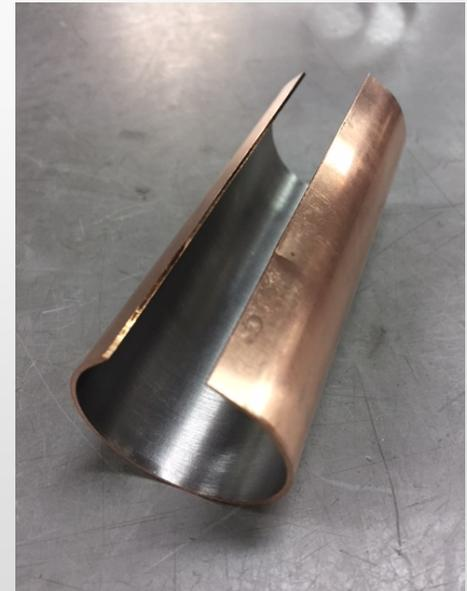
We have already successfully deposited Nb thin-film on the inner wall of Cu tube ( $\Phi 35\text{mm}$ ).
