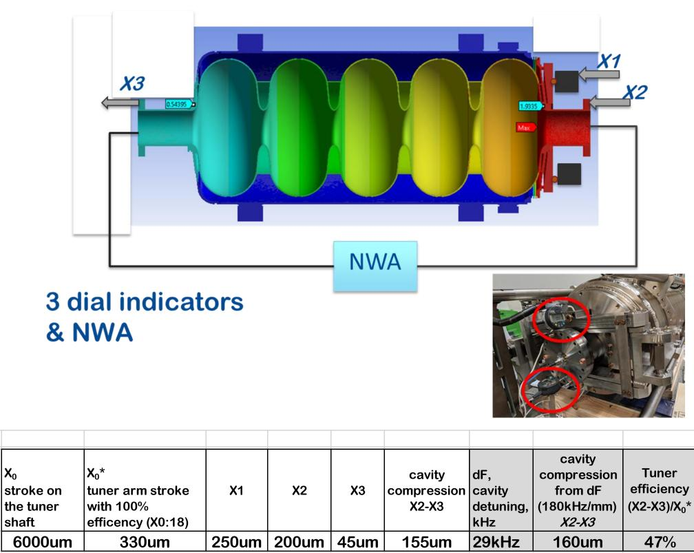
6mm/18=330um – tuning range when tuner translate 100% of the stroke to compress cavity... or k=330\*18kHz/60kStep =1Hz/step. **Efficiency of the coarse tuner ~50%**
