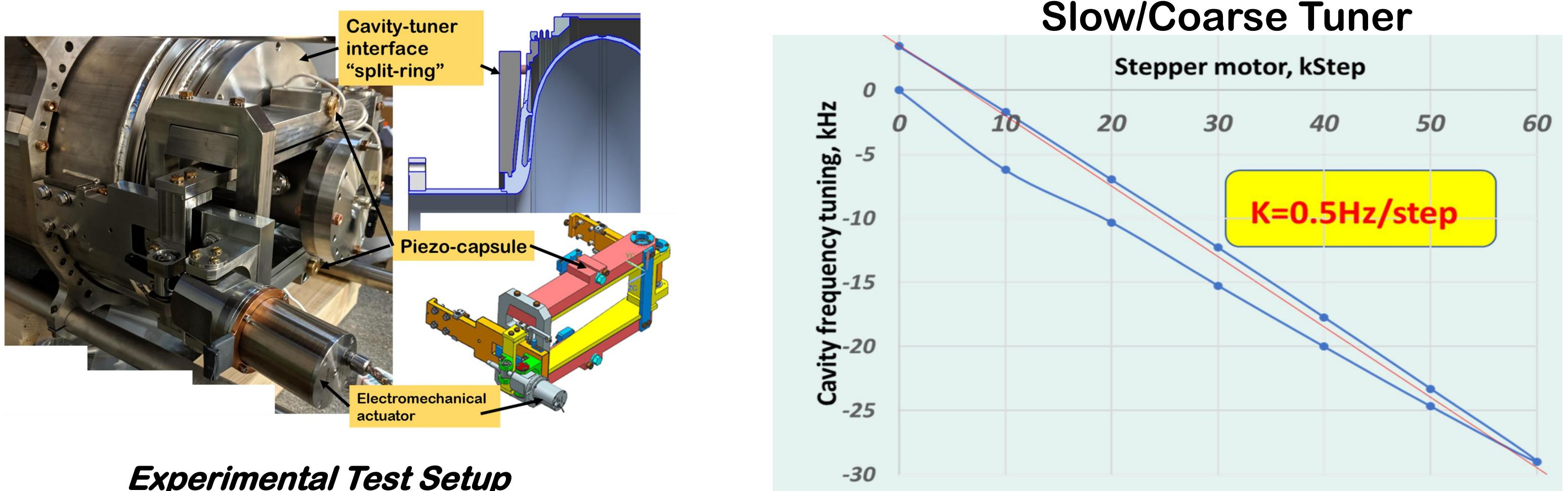
**Experimental Test Setup**
