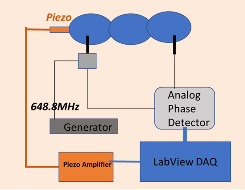
**Cavity was driven with 30** Vpp sinusoidal drive signal and frequency was stepped between 1Hz to **500Hz with increment of** 1Hz. Each sinewave (f=N Hz)
