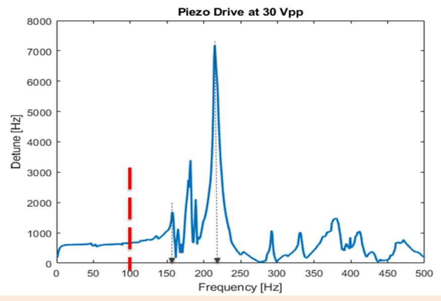
drive cavity for 3 sec and 3 second idle... to let cavity vibration attenuate before next f=N+1Hz sinevawe. **Forward and transmitted** signals feed of an AD8032 analog phase detector. **Output signal from AD8032** is proportional to the phase difference between  $P_{F}&P_{T}$  digitized at the rate of 10kHz.
