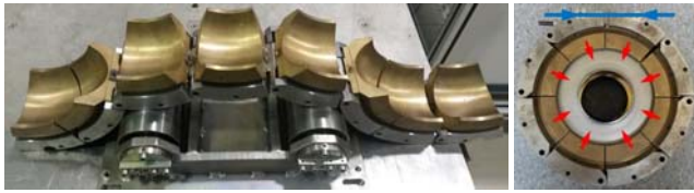
Figure 1: Reshaping chain made of stainless steel with eight brass pressing shoes (a), which distribute the radial forces (b, red arrows) by chain compression (blue arrow)
