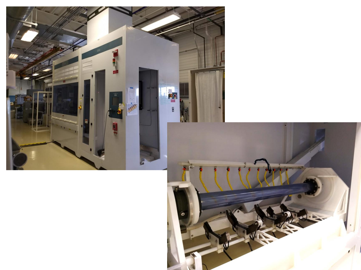
Large EP tool at FNAL CPL (top) a dummy tube was installed on EP bed for water flow test (bottom).
