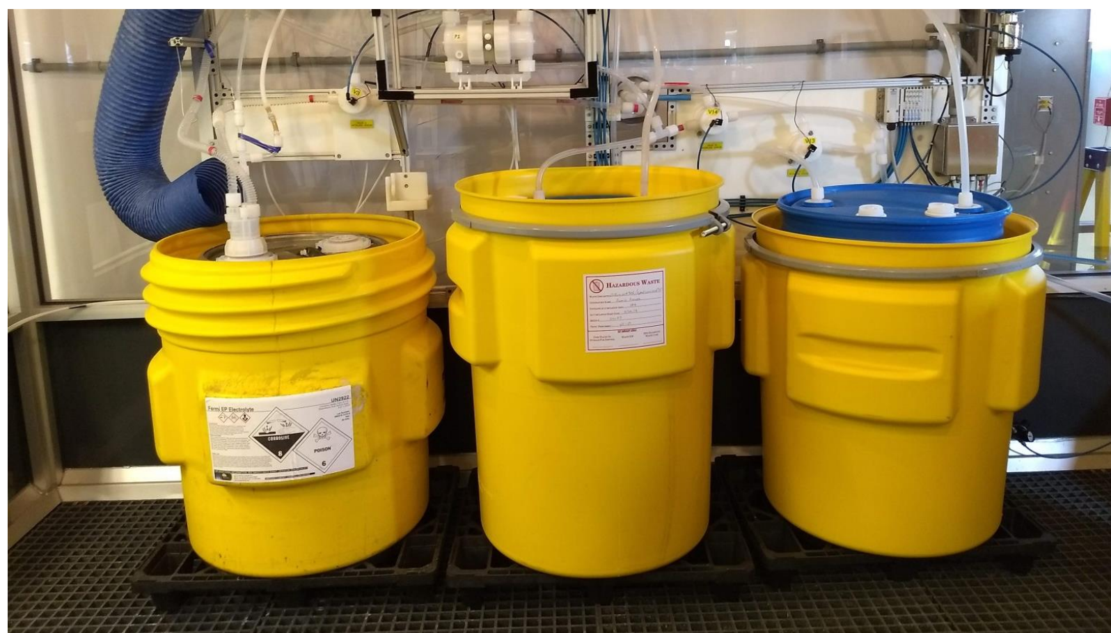
EP electrolyte drum (left) and Waste drum (middle) at chem storage room behind EP tool cabinet
