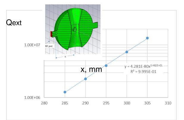
We choose fixed coupler error of ±2mm antenna position from optimum will lead increase of required Pfor of 2.5%
