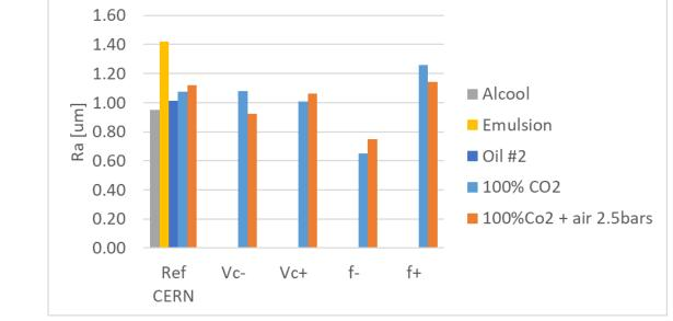
CO2 cooling allow smooth surface finish without surface contamination
