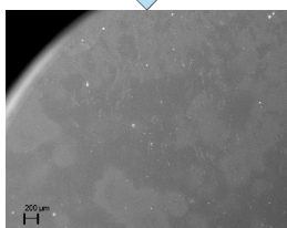
SEM image of a Nb-Pb photocathode with 2 μm Pb film with spherical extrusions which become centres of field emission.
