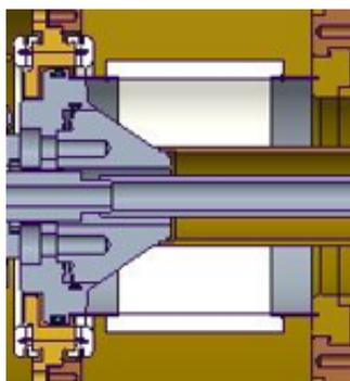
Figure 4: The new mechanical model of the cone that acts as the waveguide to coax transition, showing the split to allow for assembly.
