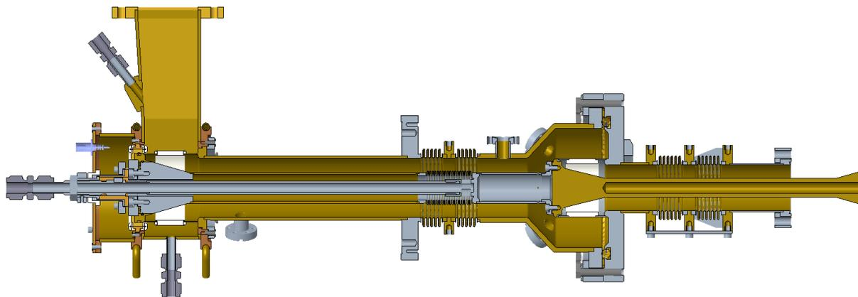
Figure 1: The finalised mechanical model of the 1.5 GHz HPC for BESSY VSR.
