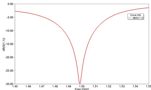
Figure 2: Plot of  $S_{11}$  for the optimised coupler.
