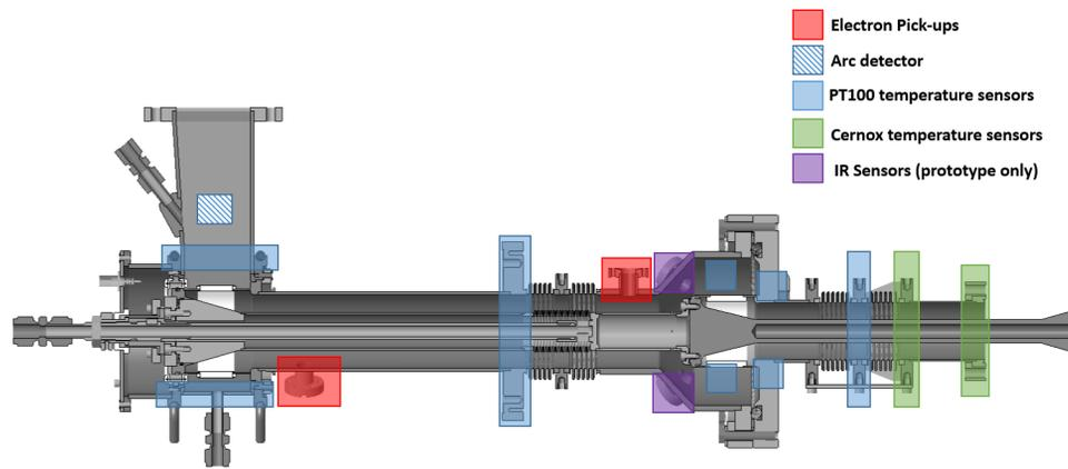
Figure 6: A view of the diagnostic prototype showing the position and type of sensors throughout the coupler.
