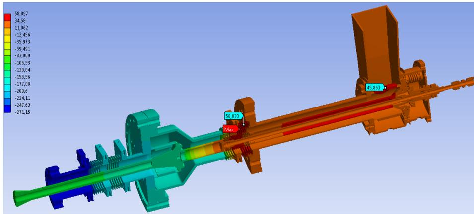
Figure 5: A temperature plot of the coupler at 16 kW operation, showing the two temperature peaks.
