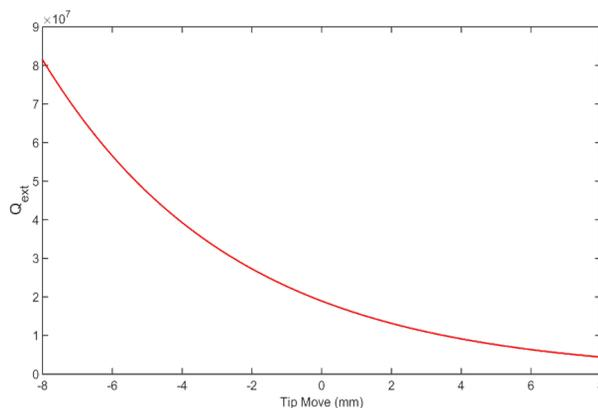
Figure 3: Plot of  $Q_{ext}$  vs Coupler tip position for an initial coupler tip design.
