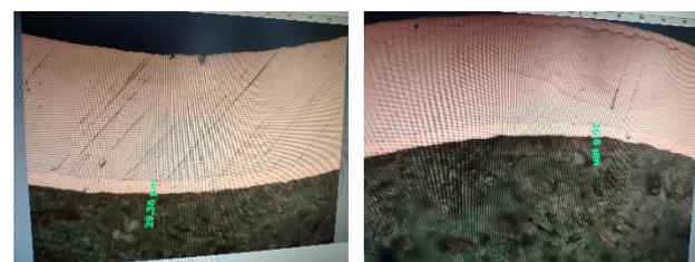
Figure 11: The measured copper plating thickness of the warm OC bellow: (a) peak: 29um; (b) valley: 26um.
