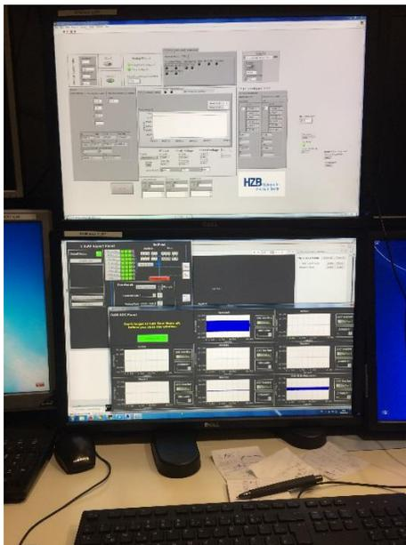
Figure 10: Virtual cavity GUI (above) and LLRF EPICS panels (below) running in the same computer of the control room.
