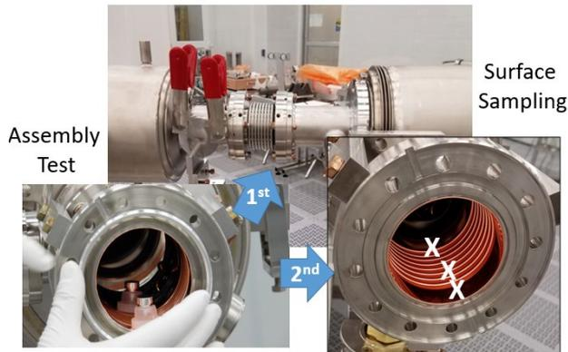
Figure 7: Particulate assessment of LCLS-II bellows assembly.
