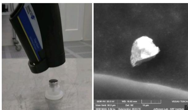
Figure 8: Particulate from N<sub>2</sub> gun test.
