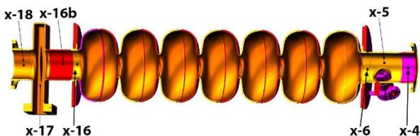
Figure 5: Sampling locations on cavities from C100-6.
