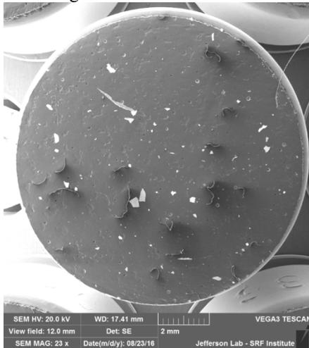
Figure 3: Sampled particulates from girder 1L12 from shaken bellows at location 13 in Fig. 2.
