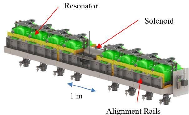
Figure 5:  $\beta=0.53$  cryomodule coldmass. Alignment rails support superconducting resonators and solenoid.
