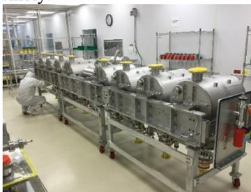
Figure 9:  $\beta=0.53$  coldmass. The coldmass is the undergoing final inspection checks prior to removal.
