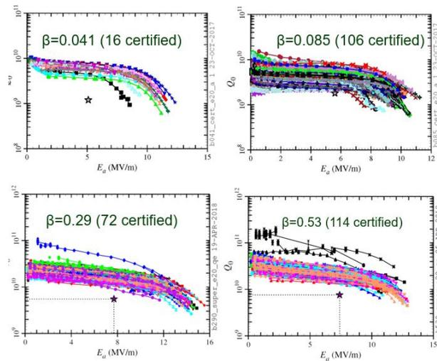
Figure 8: Dewar certification results of FRIB resonators at 2 K. Following testing the resonators are installed onto the coldmass.
