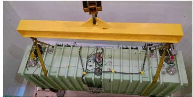
Figure 13:  $\beta=0.53$  cryomodule being lowered in FRIB shaft. After removal from the truck in FRIB loading bay, the cryomodule is lowered to the FRIB tunnel floor.
