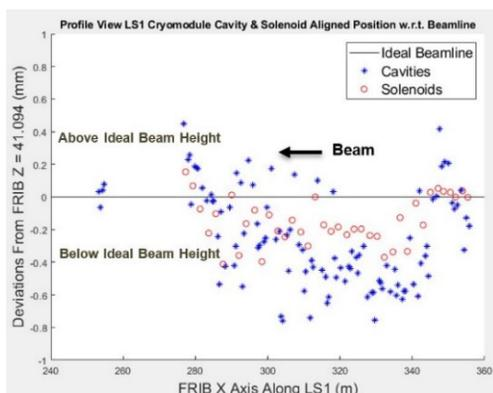
Figure 15: Profile view of calculated LS1 cryomodule cavity and solenoid as-aligned positions to the beamline.
