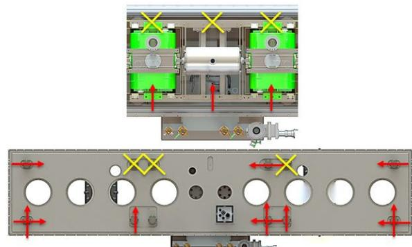
Figure 11: Cryomodule thermal contraction motion. Thermal contraction offsets are built into the cryomodule alignment.
