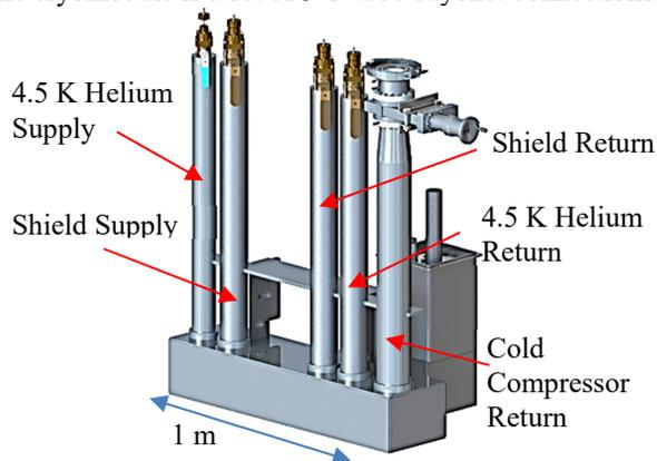
Figure 7: Cryomodule cryogenic bayonet box. The bayonet box connects to the distribution line by u-tube bayonets.
