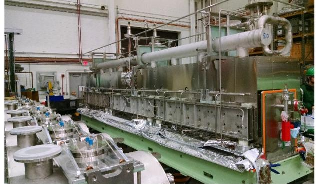
Figure 10:  $\beta=0.53$  cryomodule on assembly build floor. Cryogenic piping and magnetic shields are installed.
