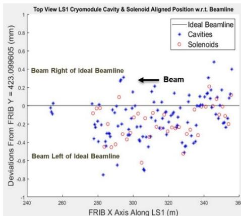
Figure 14: Top view of calculated LS1 cryomodule cavity and solenoid as-aligned positions to the beamline.
