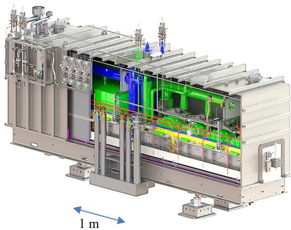
Figure 2:  $\beta=0.53$  production cryomodule bottom-up design. This cryomodule incorporates 8  $\beta=0.53$  HWRs and 1 solenoid.
