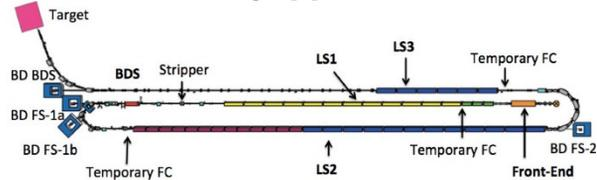
Figure 1: Schematic layout for FRIB driver linac.
