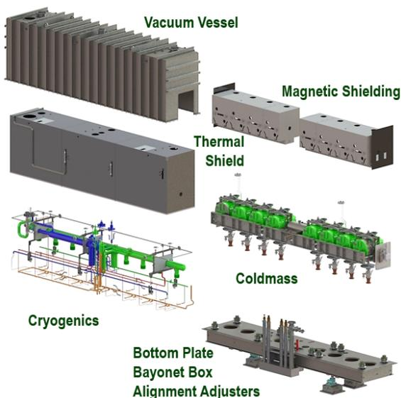
Figure 4: Sub-Systems of FRIB cryomodule design. Supported off the bottom plate is the coldmass system, where the resonators are protected by local magnetic shielding (right). The cryogenic system attaches to the coldmass. All assemblies are encapsulated by the thermal shield and vacuum vessel (left).
