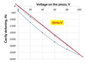
Figure 5: Cavity detuning with the piezo tuner.
