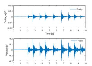
Figure 8: Amplitudes from APD and piezo (as a sensor) when cavity hit with hammer 9 times during 10 second time period.
