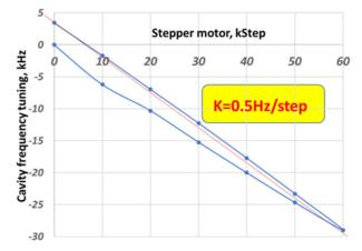
Figure 4: Cavity detuning with slow tuner.
