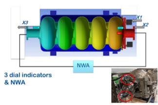
Figure 3: Schematics of the test-setup. Picture shows two (from three) dial indicators used to measure displacements of the main tuner arm and cavity beam flange.
