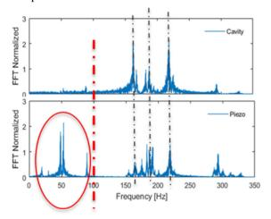
Figure 9: FFT of the signals when cavity hit with hammer (presented on the Figure 3). Top: spectrum of the cavity vibrations as measured by APD. Bottom: spectrum as measured by piezo.
