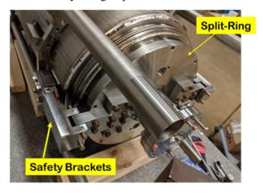
Figure 2: Split-ring and safety brackets installed on the dressed cavity.
