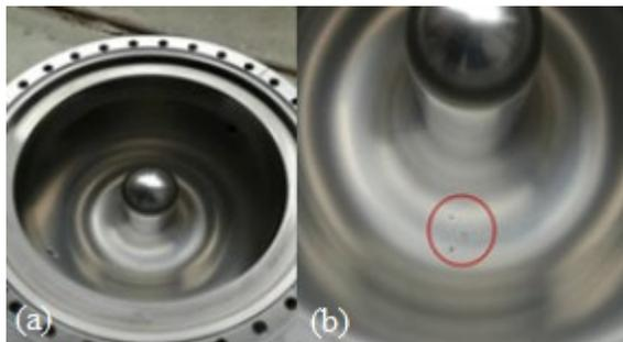
Figure 3: (a) The QWR Cu/Nb Cavity made in NIN and (b) the defects in the bottom of the cavity.
