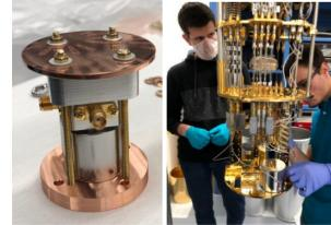
Prigure 5: 3D QWR assembly (left), attached to the 10mK stage of the dilution refrigerator at the University of Chicago (right).
