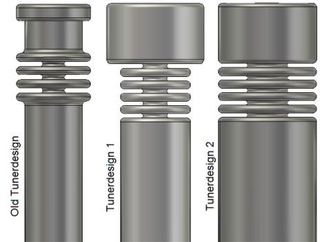
Figure 4: The three different tuner designs currently under investigation.
