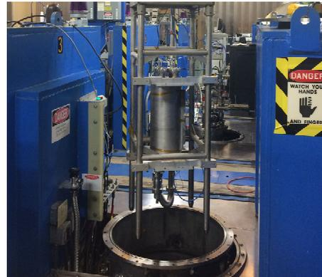
Figure 5: ODU HWR being loaded in the dewar at JLab.
