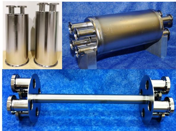
Figure 1: HWR and QWR of TRIUMF and HWR of ODU. Bottom picture is the center conductor subassembly before welding the outer conductor of ODU HWR.
