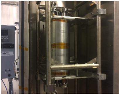
Figure 3: ODU HWR with thermocouples installed in the bake box.
