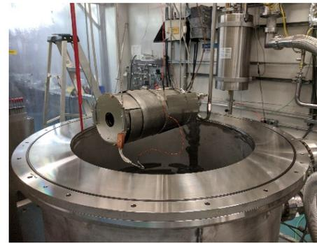
Figure 6: Loading cavity in the dewar. The QWR at TRIUMF.
