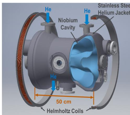
Figure 1: A schematic model of a 337 MHz HWR niobium cavity with Helmholtz coils.
