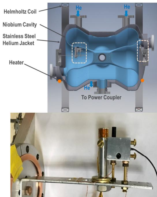
Figure 2: Cross-sectional view of the cavity model and the fluxgate installation, indicated inside the dotted rectangles (top); an actual setup of fluxgate platform (bottom)
