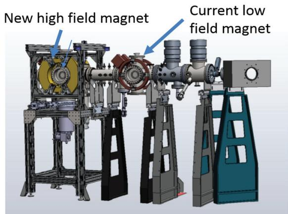
**Extension of parallel field spectrometer**
