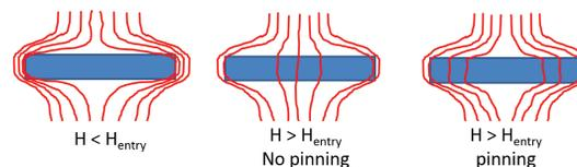
Figure 1: Left: Field breaks in at the edges first. At  $H_{\text{entry}}$  it will redistribute to the center for a pin free sample. Pinning resists redistribution requiring a higher field to reach the center.
