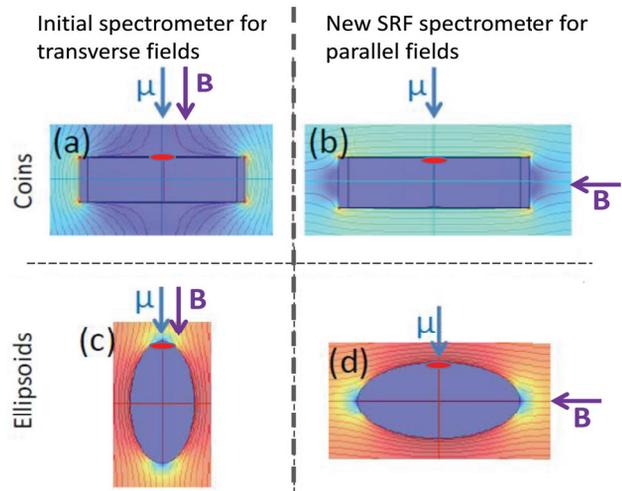
Figure 3: Four generic arrangements of sample, muon and field direction used for pinning and field of first vortex penetration studies [10].
