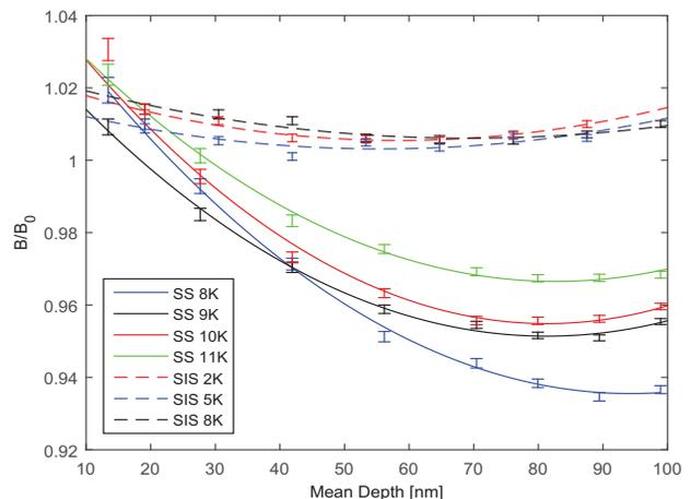
Figure 4: Field penetration in NbTiN on Nb samples with and without insulating interlayer.
