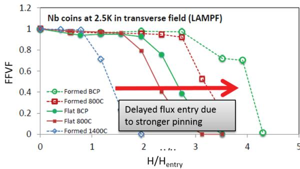
Figure 2: Field Free Volume fraction (FFVF) for a coin shaped sample with the magnetic field applied perpendicular to the sample surface.
