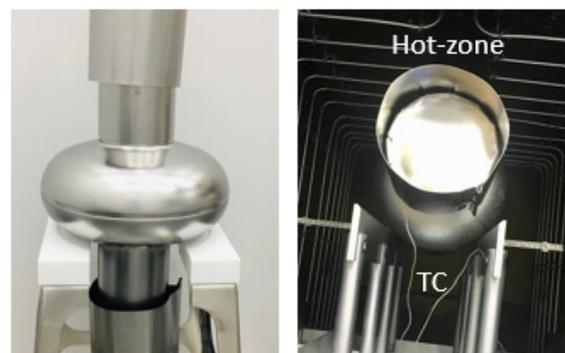
Figure 1: Installation on Nb caps in clean room (left) and cavity in furnace enclosure (right) with two thermocouples attached to cavity surface.
