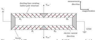
Figure 1: AMR sensor composed of Wheatstone bridge of four ferrites and aluminium barber-poles [2].
