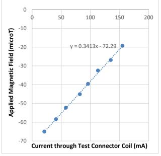
Figure 3: Cancelling applied magnetic field from a Helmholtz coil with a test coil to measure the geometry factor.
