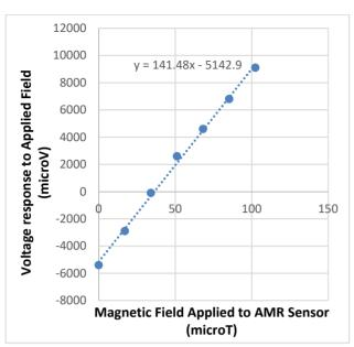
Figure 4: Sensitivity of AMR sensor at 77K.
