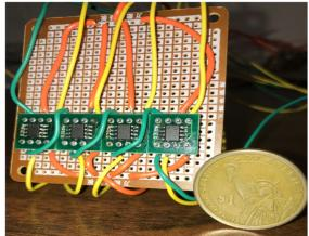
Figure 2: Four AMR sensors on a 6cm x 6cm prototype board (\$2 each).
