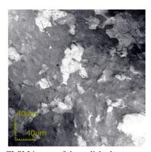
Figure 2: CLSM image of the polished copper surface following 30 mins of CP. Enhanced grain boundary etching is visible.
