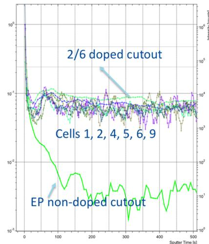
Figure 8:  $NbN^+/Nb^+$  profiles for cutouts from the equators of different cells of the 9-cell 2/0 N doped cavity showing little variation.
