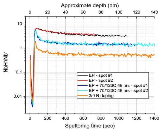
Figure 9: NbH/Nb<sup>+</sup> signal in interlaced mode for various cutouts.
