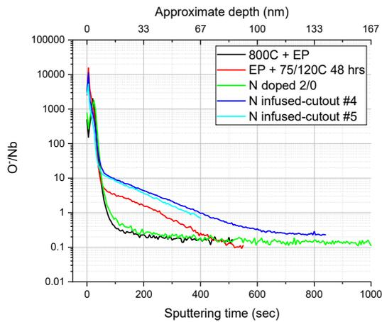
Figure 5: Oxygen depth profile comparison for EP, EP+120C, N-doped 2/0 +5 um EP, and 120C N-infused cutouts.
