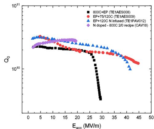
Figure 1:  $Q(E_{acc})$  curves at  $T=2K$  of the cavities used for cutout studies.
