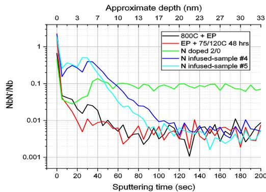
Figure 6: Nitrogen depth profile comparison between the doped, infused, and non-doped cavity cutouts.
