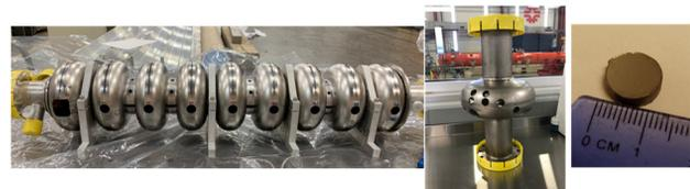
Figure 2: 9-cell 2/0 N doped cavity (left) with equator samples extracted from each cell. Single cell with cutouts from various locations and a typical sample is shown on the right.
