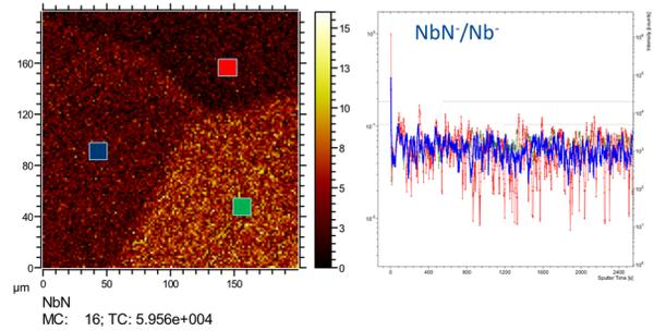
Figure 7: Comparison of  $NbN^+/Nb^+$  profile (right) for three neighboring grains (left). No concentration difference is observed.
