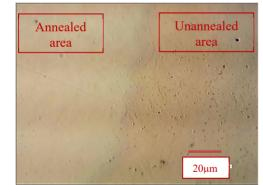
Figure 7: Metallomicroscope image of annealed Nb/Cu film. Laser energy used is 370 mJ/pulse. The defects are obviously reduced after annealing.
