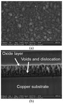
Figure 1: The SEM (a) and FIB (b) results of Nb/Cu samples deposited by dcMS [6]. It can be observed that (a) the grain size of niobium film is about several tens of nanometres, and (b) it has a network structure from the cross-section appearance and there are many voids and dislocations inside.
