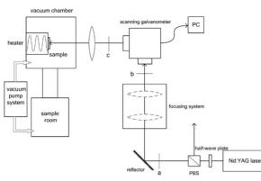
Figure 2: Sketch diagram of laser annealing system. It consists of Nd: YAG laser, scanning system, vacuum chamber and sample room.
