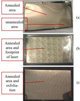
Figure 5: Effect of Nb/Cu binding force on laser annealing. (a) has the best binding force of these three samples. Scanning parameters are the same, and the laser energies are respectively (a) 352 mJ/pulse, (b) 200 mJ/pulse, (c) 300 mJ/pulse. After annealing, (a) a bright surface was obtained, while (b) and (c) both showed severe exfoliation.
