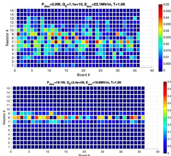
Figure 7: T-maps of CBMM-D before (top) and after (bottom) quench. Note the difference in color scale.
