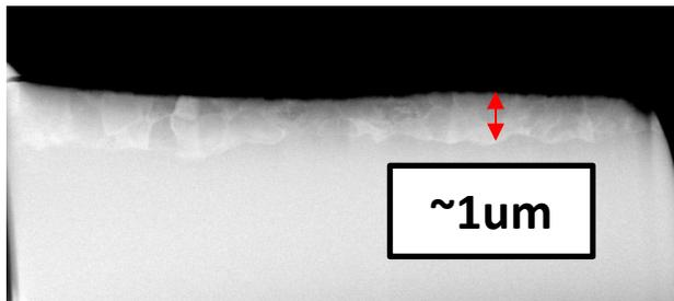
Figure 5: Measuring thickness of Nb<sub>3</sub>Sn films via a cross section extracted using a focused ion beam tool at Northwestern University.
