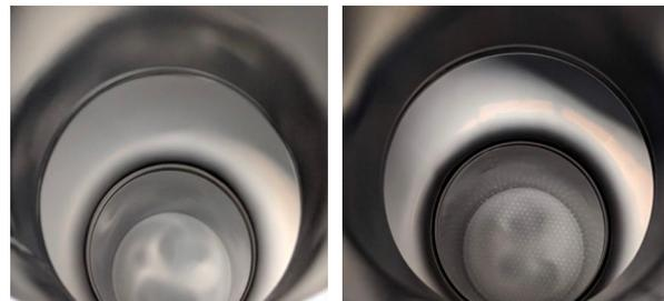
Figure 2: Typical Nb<sub>3</sub>Sn coating (left) and new Fermilab coating on CBMM-D (right), which reached 22.5 MV/m.
