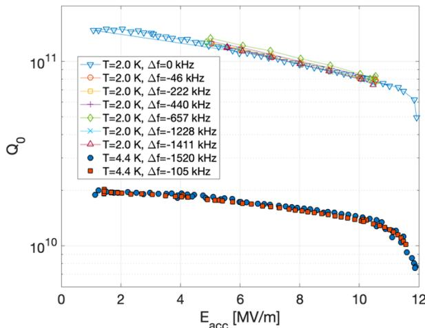
Figure 11: Results from vertical test with tuner show no effect on  $Q$  vs  $E$  at 2.0 K or 4.4 K from tuning up to 1.4 MHz.
