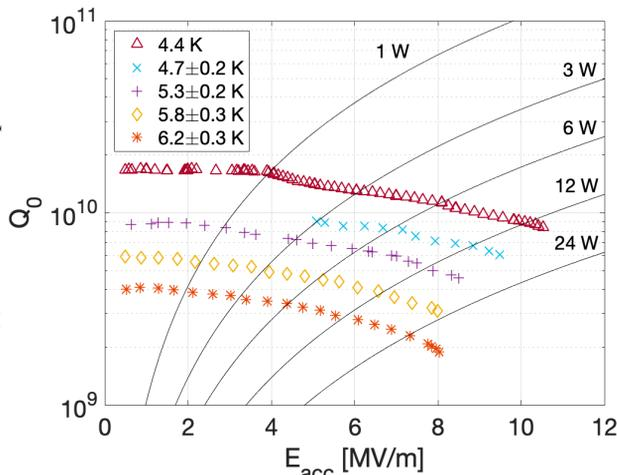
Figure 14: Comparison of the 4.4 K Q vs E curve of the 9-cell cavity to curves measured at higher temperatures in helium gas. Dissipated power curves are plotted as well.
