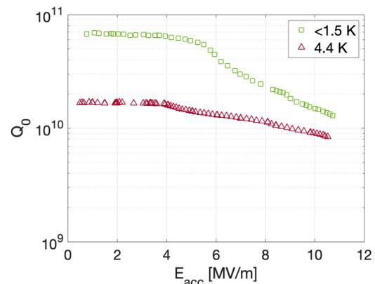
Figure 13:  $Q$  vs  $E$  curves measured at 4.4 K and  $<1.5$  K for the first ever  $Nb_3Sn$ -coated 9-cell cavity.
