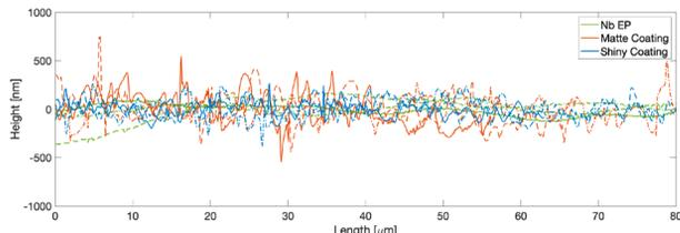
Figure 4: Line profiles of the 3 samples showing many more sharp peaks for the matte coating.
