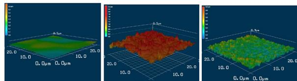
Figure 3: comparison of surface roughness of 3 samples: EP'd niobium sample before coating (left), a coating typical of previous matte Nb<sub>3</sub>Sn (middle), and a new shiny Fermilab Nb<sub>3</sub>Sn-coated sample (right).
