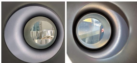
Figure 8: Pictures of the Nb<sub>3</sub>Sn coatings of the 650 MHz cavity B9AS-AES-002 from the first coating (left) with matte appearance and the second coating (right) with shiny appearance.
