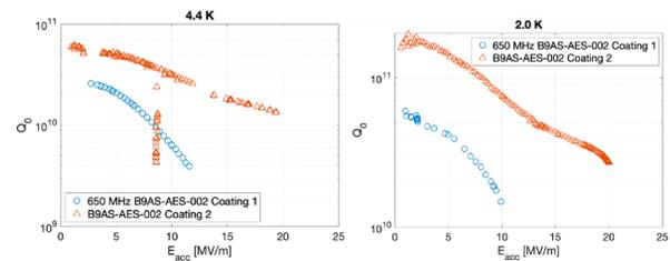
Figure 9: Q vs E curves at 4.4 K and 2.0 K for the 650 MHz cavity B9AS-AES-002 from the first coating and improved performance from the second coating. In the first coating, the gradient was power limited. In the second coating, the cavity quenched at both temperatures.
