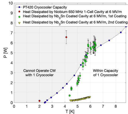
Figure 15: Dissipated power for the 650 MHz 1-cell cavity at 6 MV/m before coating, after the first coating, and after the second coating. These are compared to the capacity of a PT420 cryocooler.
