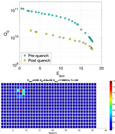
Figure 6: Q vs E curve for a Nb<sub>3</sub>Sn cavity at Fermilab before and after the first quench (top) and T-map after quench (bottom). The similar quench field after the first quench (which results in  $>1$  K heating at the quench spot) suggests that the quench is not thermal.
