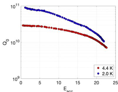
Figure 1: Q vs E curves at 4.4 K and 2.0 K for Fermilab Nb<sub>3</sub>Sn-coated cavity CBMM-D, showing a record CW accelerating gradient for Nb<sub>3</sub>Sn.
