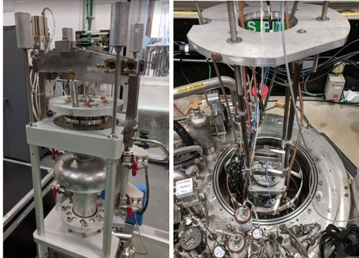
Figure 10: Setup for vertical test with tuner.
