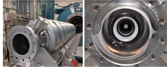
Figure 12: TB9ACC014 after coating with  $Nb_3Sn$ .
