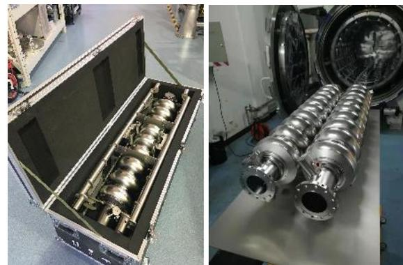
Figure 2: First FG cavity fabricated by Group-1 in the shipping box and two LG cavities fabricated by Goup-2 after 750°C annealing.
