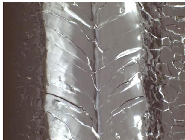
Figure 4: Photo of inner surface at one equator of FG #3 cavity, which shows no defects.
