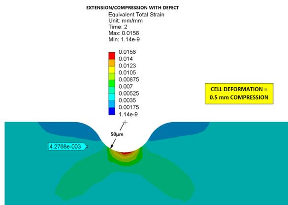
Figure 10: ANSYS tuning simulation of a smooth 50 μm groove located at the equator during -0.5 mm wall displacement. Note the higher strain levels in the pit.
