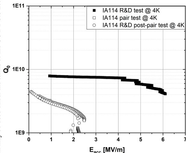
Figure 3: IA114 test results after Nb<sub>3</sub>Sn coating (full squares), after pair assembly (open squares), and after re-assembly with R&D hardware (open circles).
