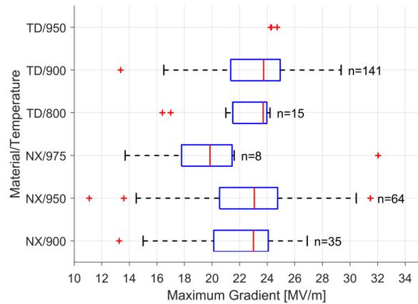
Figure 8: Quench field versus material and heat treatment temperature. Cavities treated at 975°C showed a drop in quench field consistent with furnace contamination, however statistics are limited.
