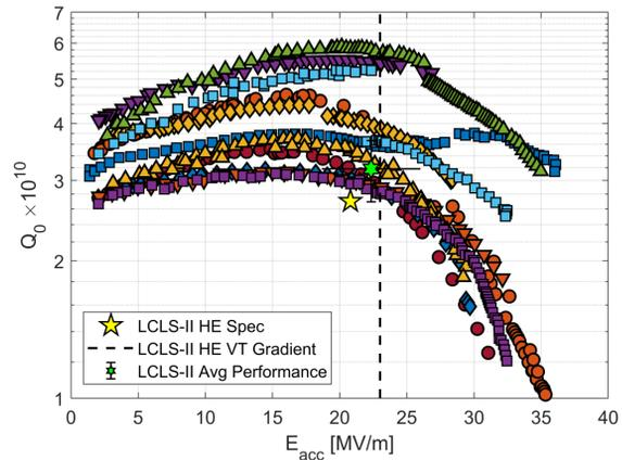
Figure 12:  $Q_0$  vs  $E_{acc}$  performance at 2 K of single-cell cavities prepared with the 3/60 nitrogen-doping. Nearly all cavities tested demonstrated performance in excess of the LCLS-II HE requirements.
