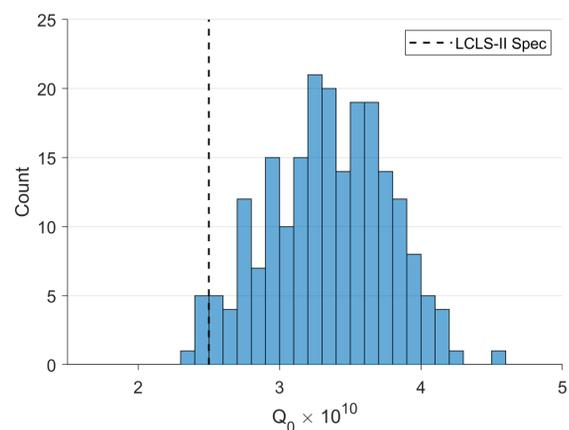
Figure 10:  $Q_0$  performance of the cavities prepared with improved fabrication procedures and heat treated at high enough temperatures for sufficient flux expulsion.
