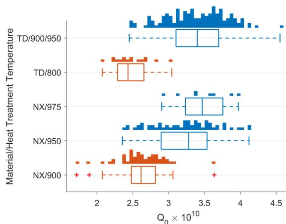
Figure 5: Boxplots and histograms showing the  $Q_0$  performance of cavities in vertical test, separated by material vendor and heat treatment temperature. TD/800 and NX/900 cavities performed poorly while treating at higher temperatures produced cavities with high  $Q_0$ .
