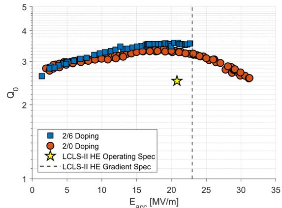
Figure 13:  $Q_0$  vs  $E_{acc}$  performance at 2 K of a 9-cell cavity produced with the 2/6 nitrogen-doping and then again with the 2/0 doping. Increase of the quench field by 30% was observed.
