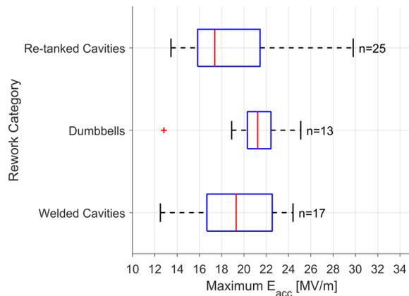
Figure 7: Gradient performance of the EZ rework cavities. Cavities that were constructed of reworked dumbbells showed the highest rates of rework success. In total ~50% of cavities were successfully reworked.
