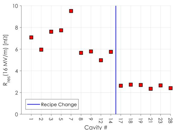
Figure 4:  $R_{res}$  of the first production cavities from RI, separated by the point in production where the degas temperature was increased from 800°C.
