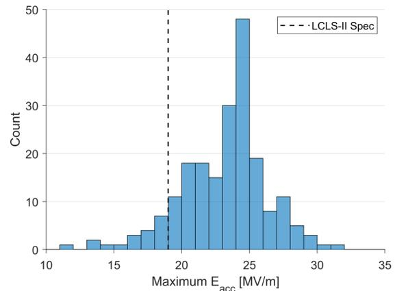
Figure 9:  $E_{acc}$  performance of the cavities prepared with improved procedures for dumbbell grinding and weld stackup.
