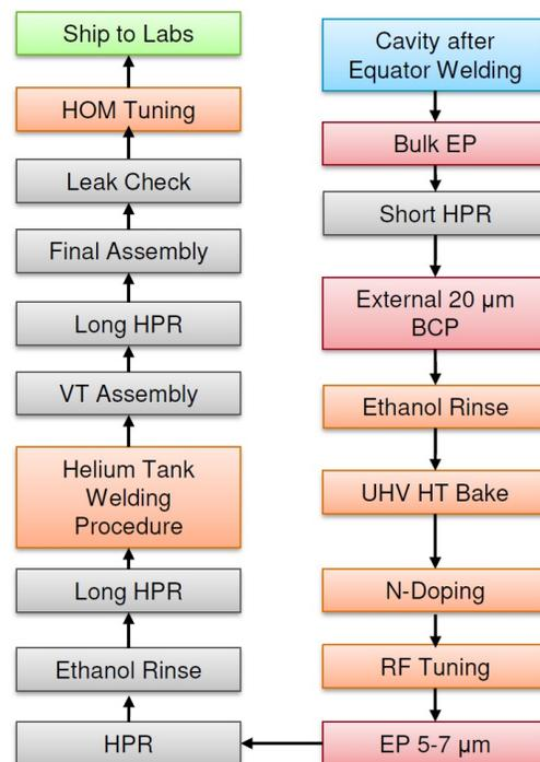
Figure 1: Production sequence for the nitrogen-doped cavities for LCLS-II.
