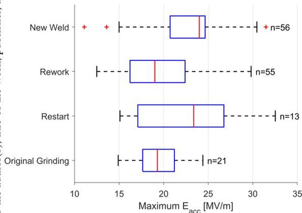
Figure 6: Gradient performance of the different groups of EZ cavities. Cavities produced with the original grinding and weld-stackup procedures had poor gradient reach. Improvement of grinding procedures led to an increase in quench fields on average but still many low performers. Rework of these cavities was marginally successful. Improvement of all procedures led to good gradient reach.
