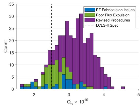
Figure 3:  $Q_0$  at 16 MV/m (or highest attainable field) for the cavities tested for LCLS-II. Also shown in the vertical test specification of  $2.5 \times 10^{10}$ . Bars are stacked.
