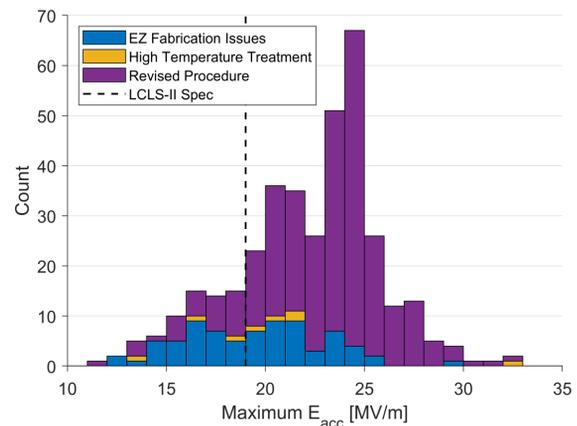
Figure 2: Maximum  $E_{\text{acc}}$  for the cavities tested for LCLS-II. Also shown is the vertical test specification of 19 MV/m. Bars are stacked.
