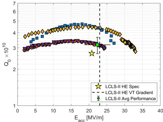
Figure 11:  $Q_0$  vs  $E_{acc}$  performance at 2 K of single-cell cavities prepared with the 2/0 nitrogen-doping. All cavities tested demonstrated performance in excess of the LCLS-II HE requirements.
