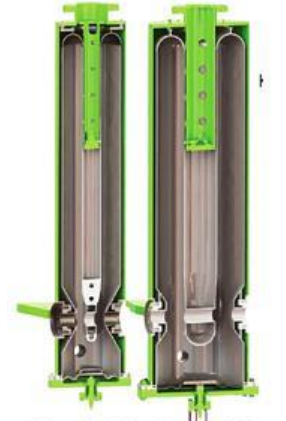
\beta_0 = 0.041 \beta_0 = 0.085 Quarter-Wave Resonators 80.5 MHz
