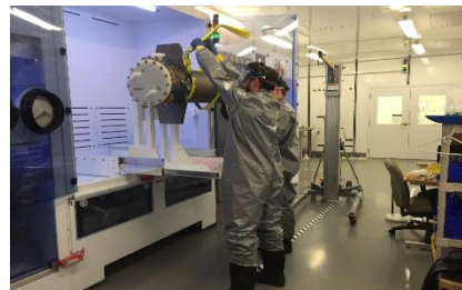
Cavity being prepared for chemical etching
