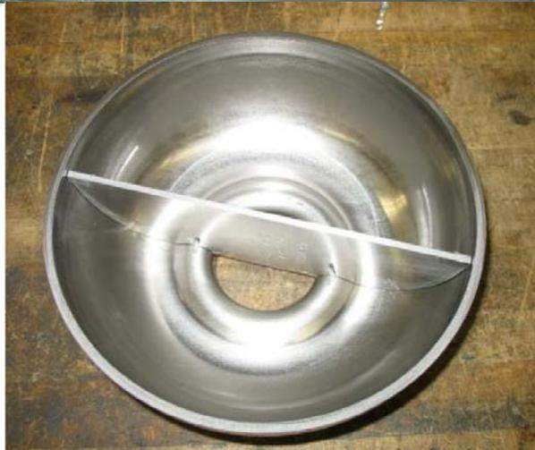
**Vent holes** were drilled in the reentrant region for both the female and male dies to **allow lubrication to escape** during stamping.
