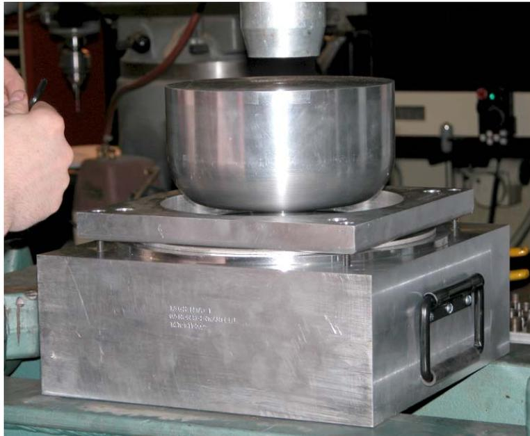
Regular two-step process: each half-cell pressed with **75 tons** followed by coining dies pressed with **17 tons**.
